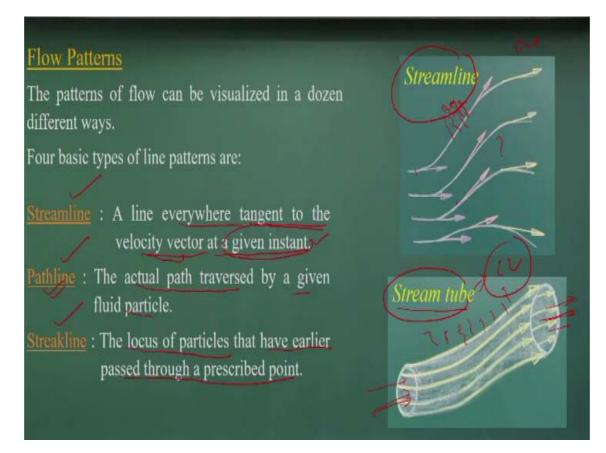
One is the streamline, pathline, and the streakline. Let us look at the definitions. The streamline, a line everywhere it is a tangent to the velocity vector at given instant. That means time equal to zero or we take a snapshot, okay. And at each point, if I draw this the tangent that tangent should give a directions of the velocity vector okay. So if you look at this that as I draw this, these tangent line, this line tangent should match with the directions of the velocity.
