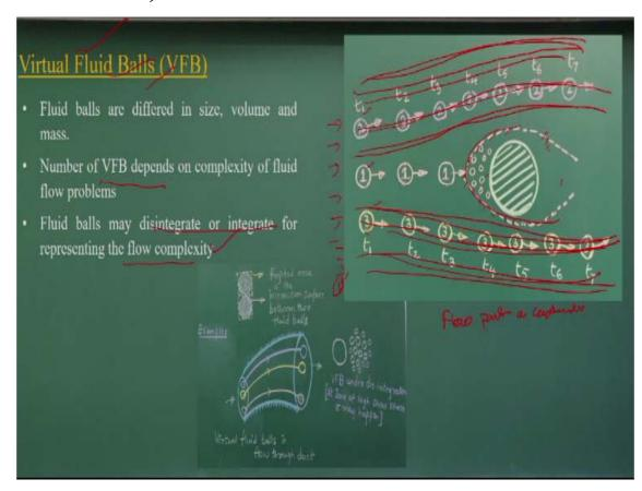
The for example, if I take these problems that flow passed a cylinder. That means I have a cylinder, a velocity of v uniform velocity of v is passing through this. okay? As I told it earlier I will have a virtual fluid balls okay it is not real fluid balls these are virtual fluid balls. I have a ball 1, 2, and 3 and this is the fixed. And these balls are having a velocity v as equal to the velocity of uniform flow.
