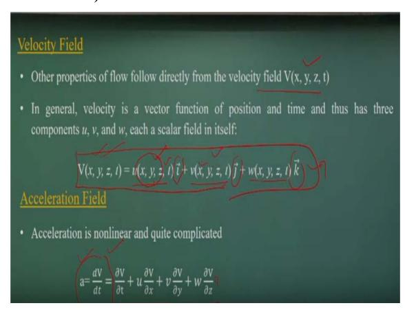
So now I am just defining them the velocity field, when we are talking about we are talking this velocity as a vector quantity, which vary in a space in case of the Cartesian coordinate system of x, y, z and the time. But most often for easy point of view, we resolve this velocity vector component into its scalar component in Cartesian coordinate systems like the i and j and k.
